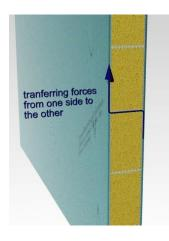
A sandwich construction made with **FiberPlank**<sup>®</sup> is much stronger than a normal balsa-core ore foam sandwich construction. This is because of the 'bridge' connection between both of the outside reinforcement layers, which enables forces to be transferred from one side to the other and vice versa. This bridge also provides a very high level of resistance against compression forces.
