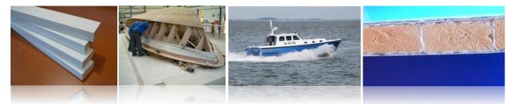
Applying **FiberPlank**<sup>®</sup> is both simple and efficient. Simply construct a panel by bonding the strips side by side, using epoxy. Then laminate an enforcement layer on both sides. The enforcement layer could be E-glass, carbon fibre, aramid or any other kind of modern reinforcement fibre.
